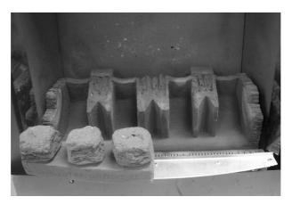
c) Place the right hand front coal rail moulding onto the front ceramic rail support as shown below in Fig. 3
