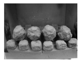
e) Select three of the small coals and fit onto the ribs of the fuel-bed base. See fig. 5 below
