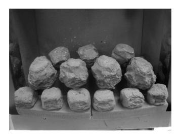
f) Select the remaining four small coals and arrange along the rear of the fuelbed, directly behind the third row of coals. See fig. 6 below.
